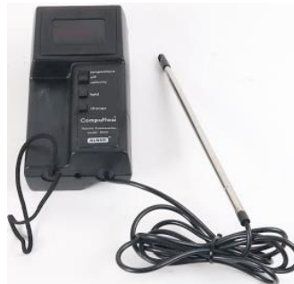
Figure 4: ALNOR CompuFlow 8525 Thermal Anemometer
