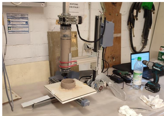
Figure 3: 3D printing with salt-clay mixture.
