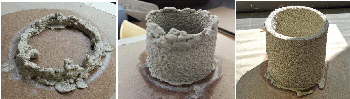
Figure 4: 3D printed Cylinder. From left to right: Material mixture with insufficient water content, material mixture with excessive water content, material mixture with optimal proportions of components (Photo: EBB TUM).
