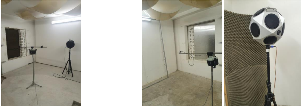
Figure 3: Positioning of the audio-acoustic equipment in Room 1 (left) and Room 2 (right).
