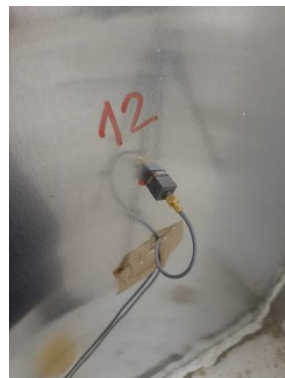
Figure 4: Mounting the accelerometer on the aluminum layer.
